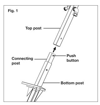
2. Slide the top post over the connecting post until the push button locks into place in its respective hole on the top post (Fig. 2).
